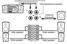
If you have connected external side speakers to the television, set the internal/external selection button (located at the rear of the television set close to the connectors) to the external position (pushed down). Use the point of a pen.
